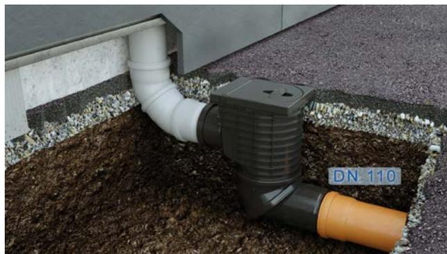
With curtain walls the downpipe very often is hidden between the brick wall and the curtain facade. In this case a normal rain hopper may not be used, as the opening of the lid no longer is possible. Beside of that there has to be a watertight connection between downpipe and rain hopper. We have got the solution: HL600NHO! With all advantages of the new rain hopper HL600N, but with a watertight socket connection DN110!
